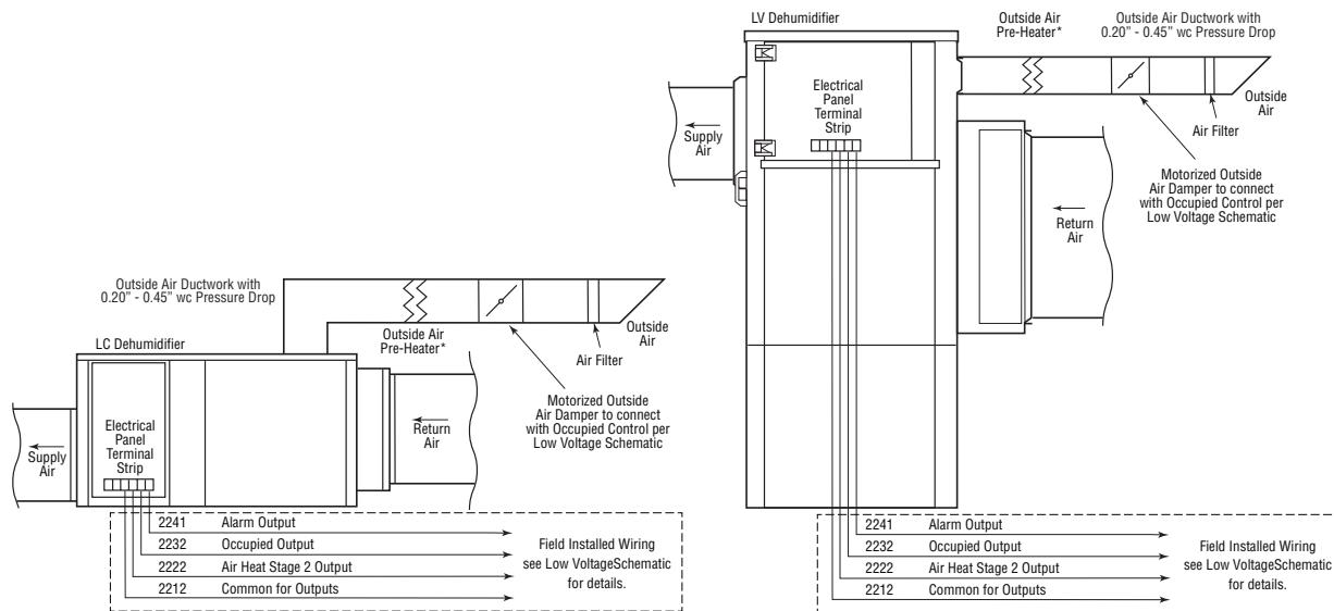
Figure 34 - Proper Installation for an Outdoor Air Application
