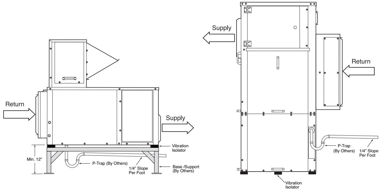
Figure 26 - Condensate Piping
