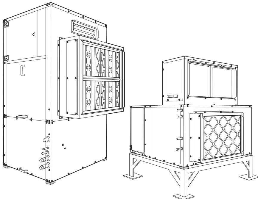
*Figure 21 - Typical Floor Installation*
