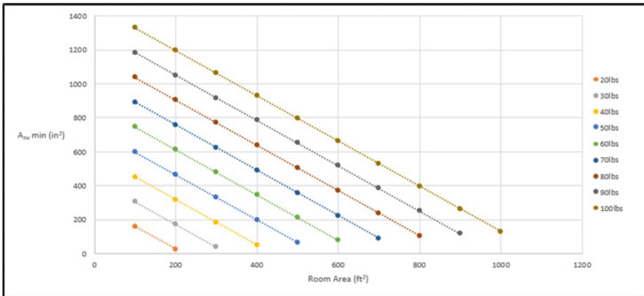
Figure 4: Chart GG.7 - Required Opening ( $in^2$ ) per Given Room Area ( $ft^2$ )
