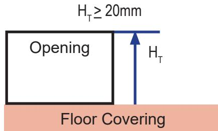
Figure 8: Minimum Height Requirement for Floor-Extending Openings
