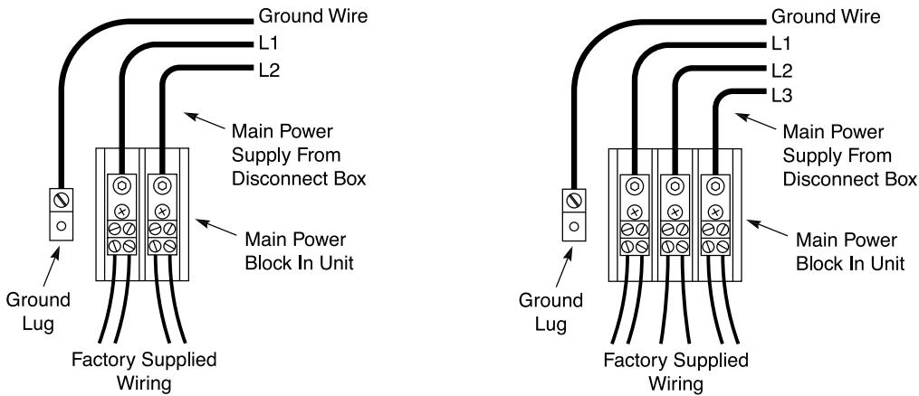
Figure 30 - Single-Phase and Three-Phase System Power Connection
