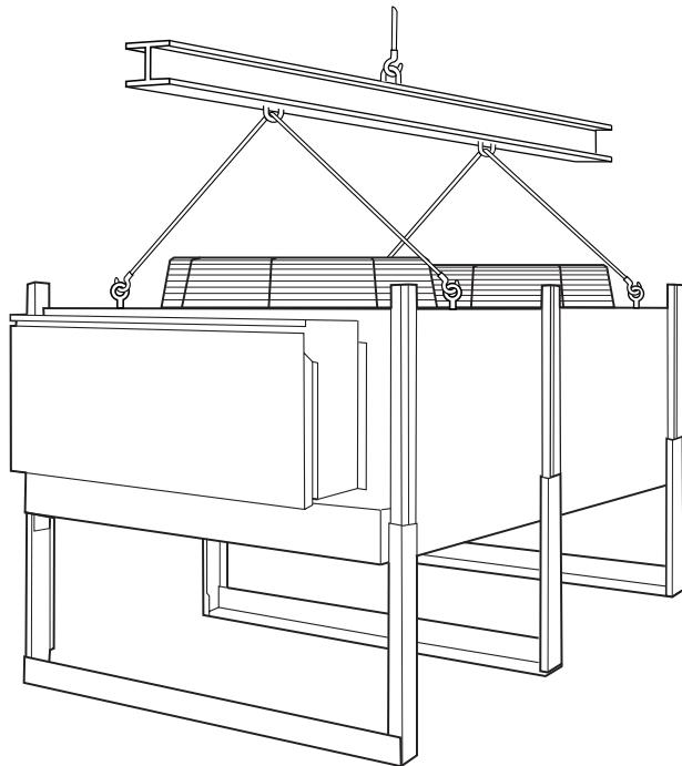
*Figure 20 - Typical Rigging for an Optional Remote Condenser*
