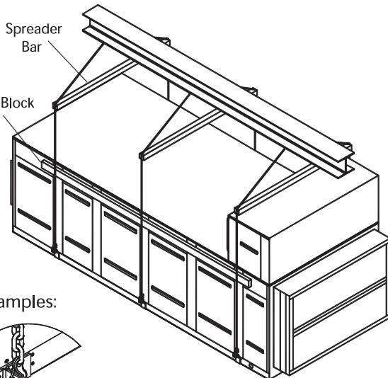
Figure 19 - Typical Rigging for Large Systems
