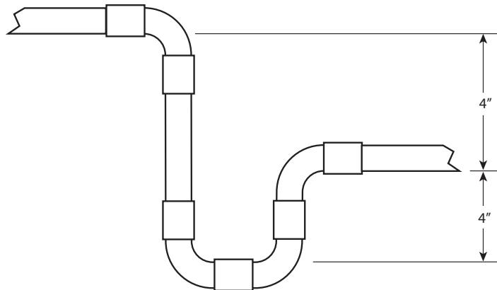
Figure 27 - Sectional View of Condensate Trap Requirements
