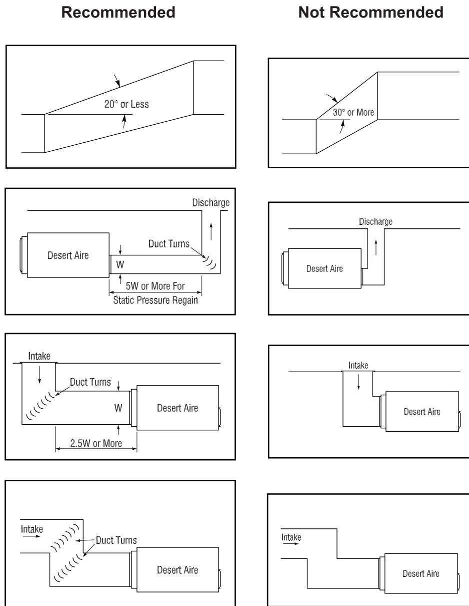
Figure 40 - Recommended Duct Designs for Desert Aire dehumidifiers
