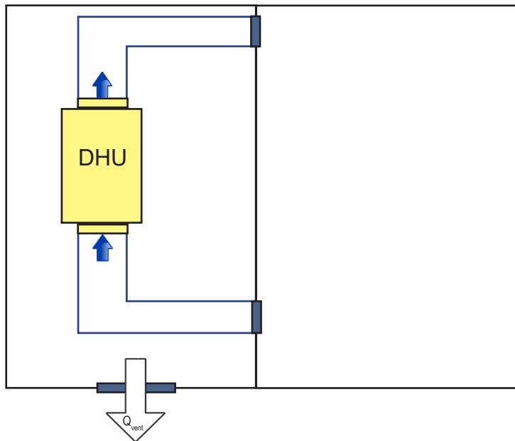
Figure 18: Mechanical Ventilation of Machinery Room to Outdoors
