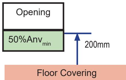
Figure 6: Minimum Natural Ventilation Opening Requirements Below 200mm
