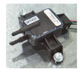
Figure 3 - Pressure Transducer in Electrical Box
