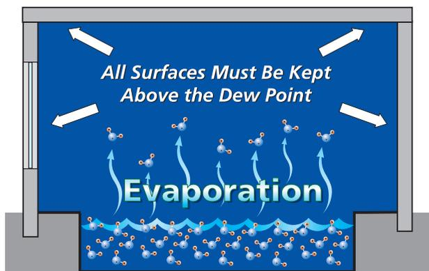
Figure 1 - Proper Dew Point of Pool Room Surfaces
