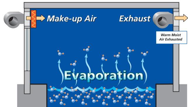
Figure 2 - Make-Up Air / Exhaust Method
