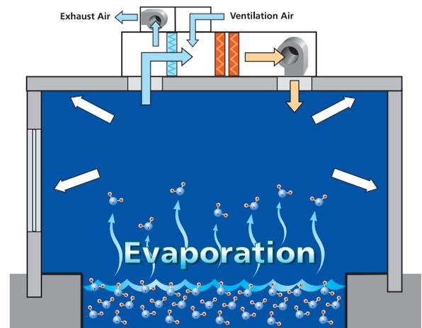
Figure 3 - Refrigeration-Based Dehumidification System
