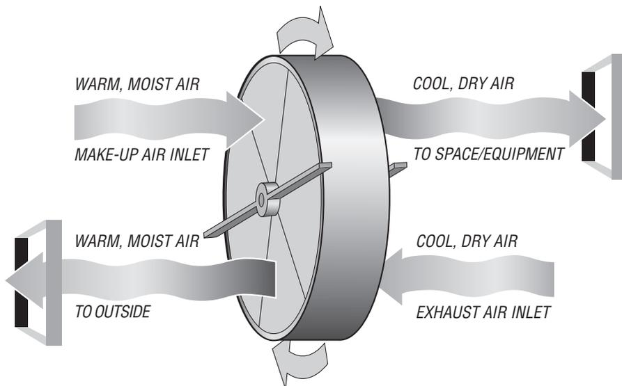
Figure 1 - Typical Enthalpy Wheel Operation (summer operation)
