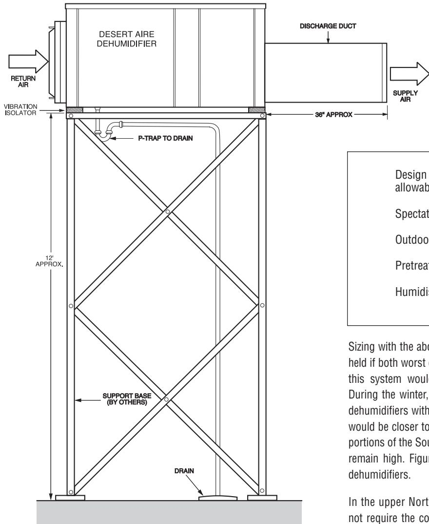
Figure 4 Dehumidification System Installation
