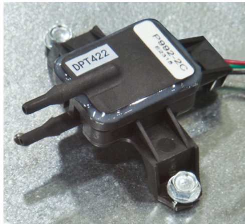
Figure 3 - Pressure Transducer in Electrical Box
