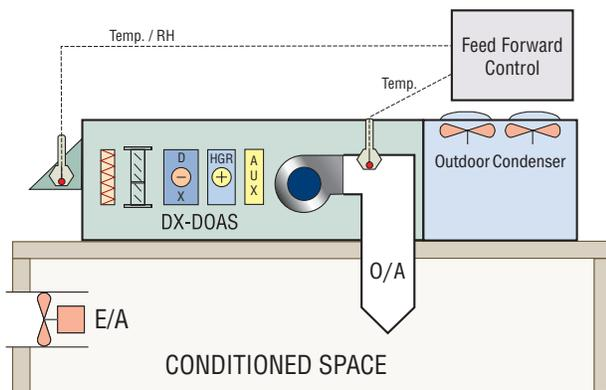
Figure 2 - Outdoor Air Reset Control Configuration
